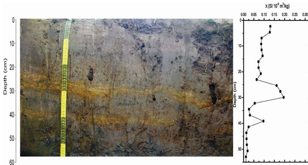
Figure 2. Detail of Ixt-048 trench showing stratigraphy and magnetic susceptibility data. Dash lines bound events 1 and 2.
