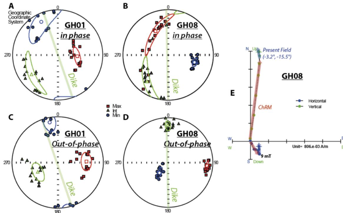
**Figure 3.** A-B. In-phase AMS for samples GH01 and GH08. C, D. Out-of-phase AMS for samples GH01 and GH08. E. Zijderveld diagram of an AF demagnetization (GH08).
