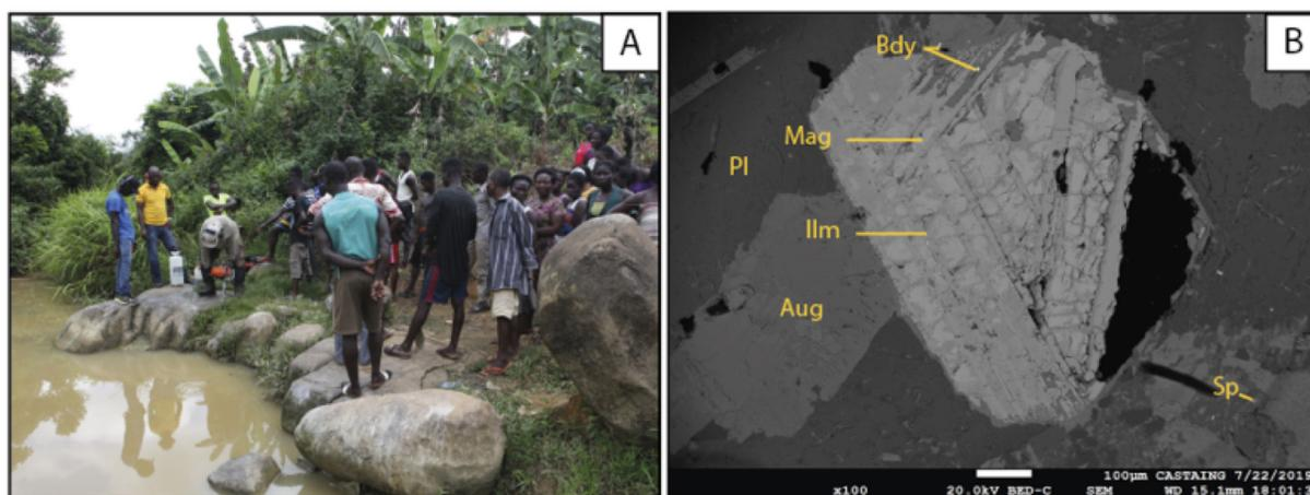
**Figure 2.** A. Sampling of a well *in situ* Manso dike (GH08). B. BSE micrograph of titanomagnetite (Mag) with exsolutions of ilmenite (Ilm), augite (Aug), plagioclase (Pl), spharelite (Sp), and baddeleyite (Bdy) (GH09).
