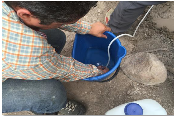
Colecta de gases Giggenbach
