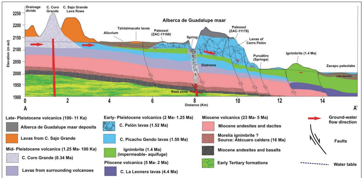
Figure 9: SE-NW profile cutting through the Alberca de Guadalupe maar showing the observed and inferred geological units (as indicated in Fig. 8) and horizontal groundwater flow direction (red arrows). Taken from Kshirsagar *et al.* (2015).
