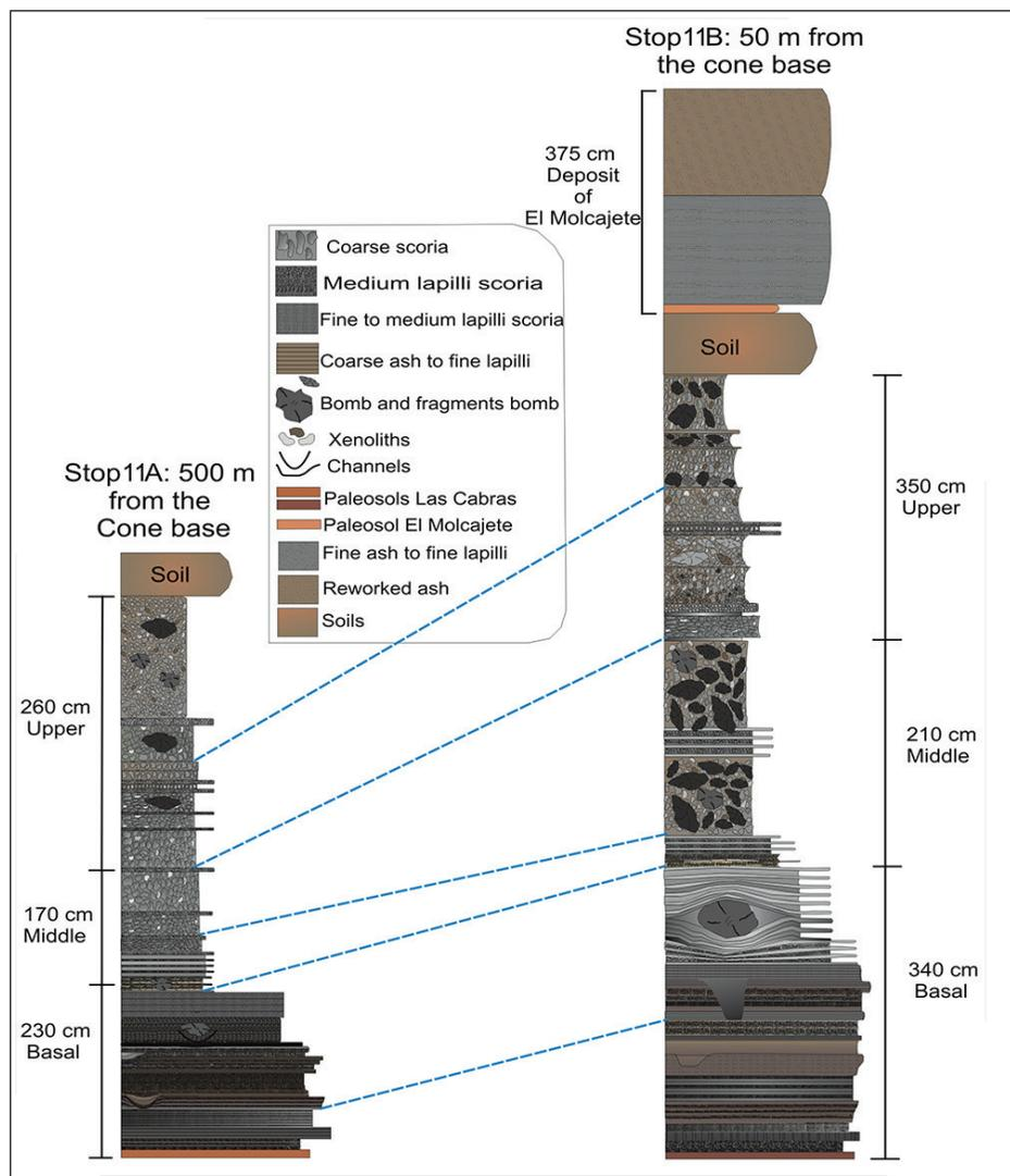
**Figure 39: Stratigraphic sections of Las Cabras fallout deposits at Stop 11A located 500 m and another quarry (Stop 11B) located 50 m from the base of the cone. The different parts of the sequence (basal, middle, upper) described in the text are indicated. Layers at the most proximal quarry are thicker, richer in bombs, and contain larger bombs in the upper part. Taken from Siebe *et al.* (2014) and drawn by Athziri Hernández.**
